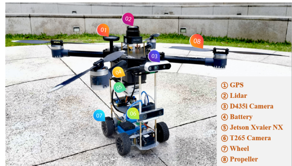
Fig. 5: The detailed composition of our customized air-ground robot (AGR).
